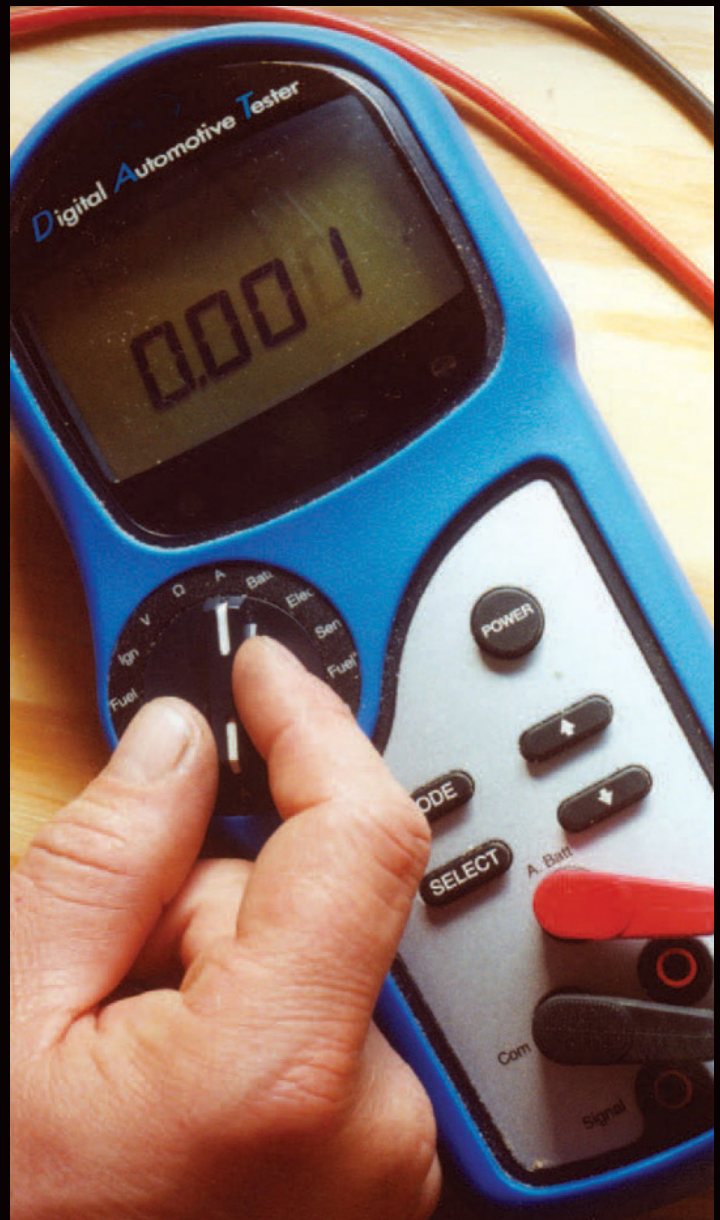
Your DMM should have a voltage bar scale to make it useful in checking oxygen sensor output, but a graphing multi-meter, or a lab scope would give you better information.
