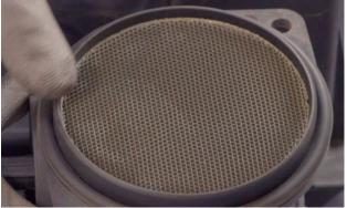
WALKER PRODUCTS DOES NOT RECOMMEND USING MASS AIR FLOW CLEANER AEROSOL SPRAY. DOING SO COULD DAMAGE THE MASS AIR FLOW SENSOR.
