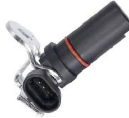
WALKER # 1008-1011 CRANKSHAFT POSITION SENSOR 1998-2002
