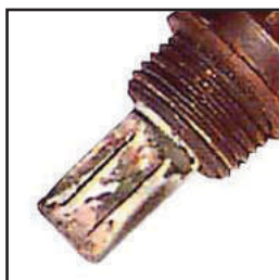
Ethylene Glycol (Antifreeze) Contamination
