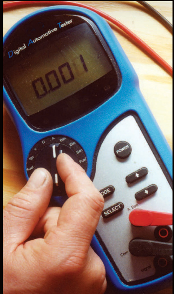
Your DMM should have a voltage bar scale to make it useful in checking oxygen sensor output, but a graphing multi-meter, or a lab scope would give you better information.
