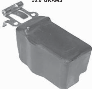
100-70 KEIHIN REPLACEMENT FOR HONDA 16013-657-005, 16013-657-015 10.0 GRAMS
