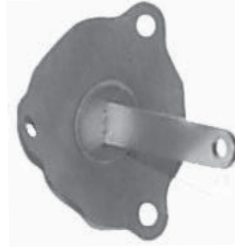
745F (W-2) (CHOKE PULL-OFF DIAPHRAGM) RENAULT (4) 1981
