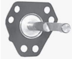
389F (SL-1) (CHOKE PULL-OFF DIAPHRAGM) VOLKSWAGEN (4) 1972-74
