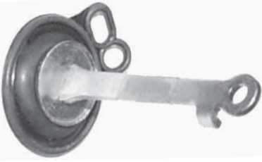
1046F (MI-SL) (CHOKE PULL-OFF DIAPHRAGM) CHRYSLER IMPORT (4) 1980-86 MAZDA (4) 1980-86 MITSUBISHI (4) 1980-86
