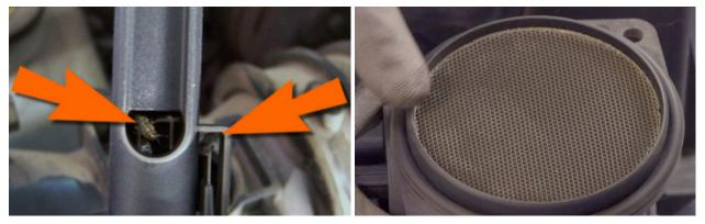
WALKER PRODUCTS DOES NOT RECOMMEND USING MASS AIR FLOW CLEANER AEROSOL SPRAY. DOING SO COULD DAMAGE THE MASS AIR FLOW SENSOR.
