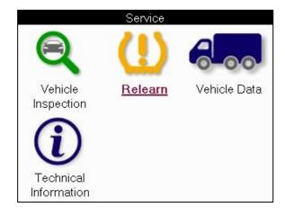
To find out which relearn type is available for a vehicle, just turn on the tool and select Relearn. Or refer to the current coverage list at www.bartecautoid.com > Downloads.
