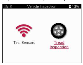
The selected wheel and tread position will be highlighted on the display. Press the enter key to enter the tread manually, the valid input range is 0-32/32<sup>nds.</sup> Repeat this for each wheel and position: outer, centre and inner if using 3 tread measurements. The number of tread measurements to input can be changed from 1 to 3, with 3 being the default. The number of readings and the measurements can be configured in the Tread Settings.
