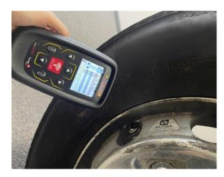
(Note: with Ford Banded sensors the tool should be held 180°/opposite from the stem's position)
