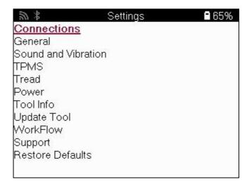
Connect to a Bluetooth OBDII Module, TPMS Desktop, and Wi-Fi.
