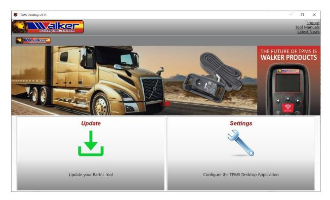
Connect the TECH600 to the computer. The TPMS Desktop will automatically register the tool and will display the message: "Tool successfully registered". The TPMS Desktop will then check for any updates that can be applied to the tool. Alternatively, the user can navigate to 'Update.'
