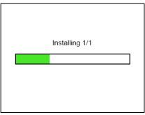
Please do not disconnect the OBDII module from the vehicle, turn off the TECH600, or otherwise stop the installation of the update while this screen is displayed.
