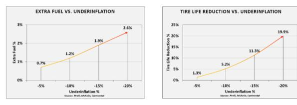
With Walker TPMS sensors, you can expect more accurate readings thanks to their increased measurement frequency compared to OE sensors. This precision translates into better fuel mileage and reduced tire wear, leading to significant cost savings over time. Additionally, Walker sensors go beyond pressure monitoring by measuring tire temperature, allowing telematics systems to predict potential tire blowouts and prevent accidents.
