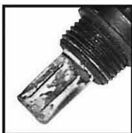
Ethylene Glycol (Antifreeze) Contamination
