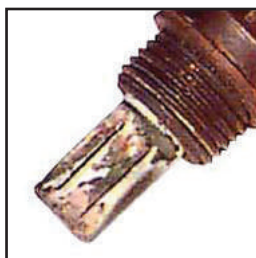
Ethylene Glycol (Antifreeze) Contamination
