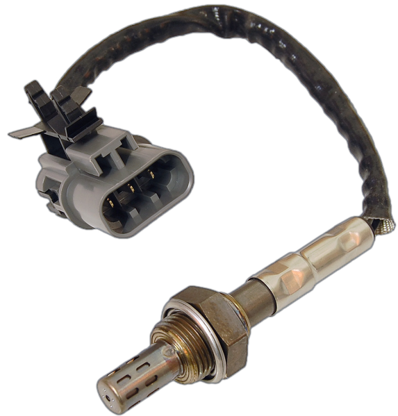
This is an older three-wire HEGO (Heated Exhaust Gas Oxygen) sensor. The black wire carries the signal.
